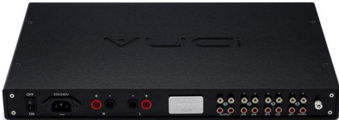
The amplifier's chassis is a good strong rigid affair made from aluminium and a nice touch is the recessed stainless steel screws which won't rust or distort the first time you need to take the lid off (not that you would). Talking of chassis and lids, note there are no ventilation holes or slots in same, as the
